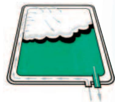
Forced air removal design with combined purging
