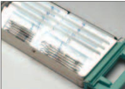
Wrapped instruments arranged with drying plates (STAT/M 5000)
